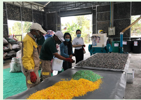
PatiHoub factory staff sort and arrange the shredded plastic for the design of the board before it is pressed. Luang Prabang, Lao PDR (June 2024)
